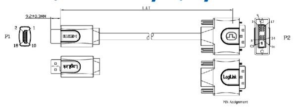
Our DVI to HDMI cable is specially designed for connecting your computers DVI output into your hi-def Plasma or LCD TV. We use premium grade material for our cable components and jackets. Our gold plated connectors ensure better connectivity, signal strength and cable-life longevity. Our DVI to HDMI cables are bi-directional, so you can send a signal from HDMI to DVI too. Set up your Multimedia Center like a professional, with the high quality cables you expect from us.
